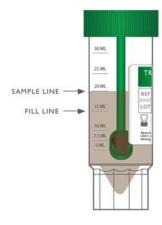
Add 5g of sample to the vial, bringing the level to the sample line.
