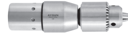
M208-309 Drill attachment with keyed chuck Ø4 mm Cannulated Ø 1.0 mm - 6.35 mm 900 rpm / 4 Nm 30 x 126 mm / 370 g
