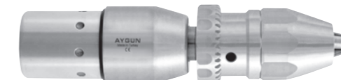
M208-313 Drill attachment with hybrid chuck Both keyed and keyless operation Ø4 mm Cannulated Ø 0.3 mm - 3 mm 900 rpm / 4 Nm 30 x 130 mm / 395 g
