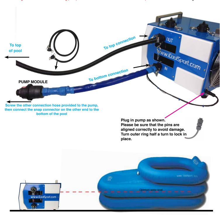
The iCool must be on the same level surface as the pool. It must not be above the pool. The pump must be on the floor and lower than the water in the pool. The water level in the pool must be well above the pump and the hose pipe with the pump must be flat on the floor to prevent air being trapped.
