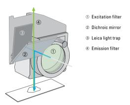
Several newly developed fluorescence filter systems for LMD allow the unique simultaneous cutting under fluorescence:
