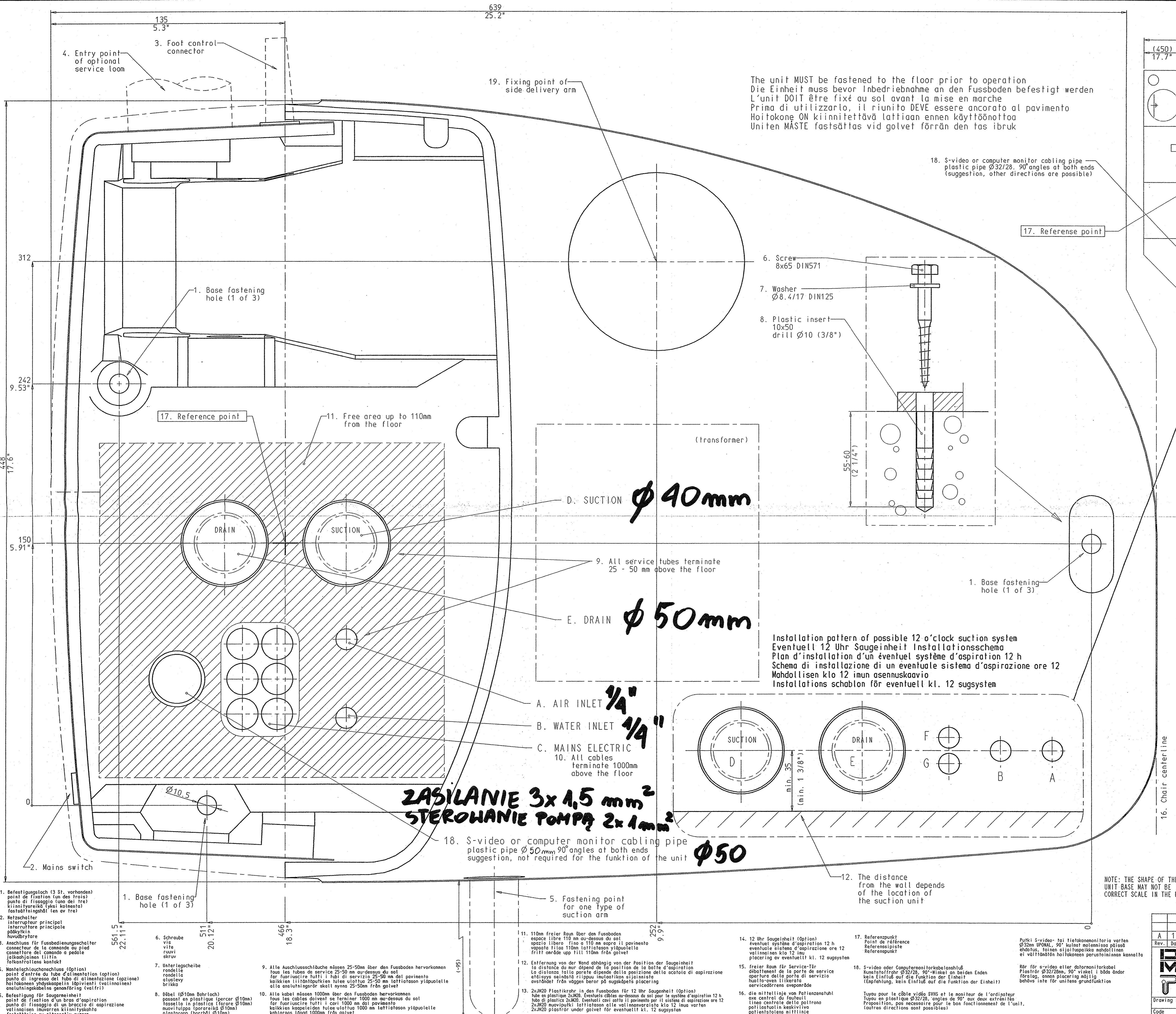
The unit MUST be fastened to the floor prior to operation
