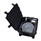
1921046 NESTED HEAD AND BODY CT PMMA KIT IN STORM CASE
