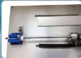
Fix the trocar with the jig. It means the test is ready.
