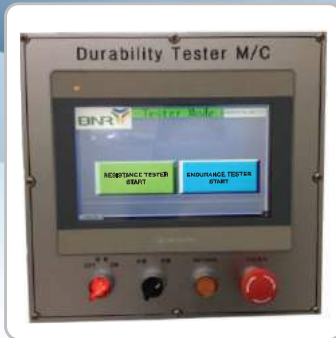
You can choose 'Resistance test' or 'Durability test' with touching the screen.
