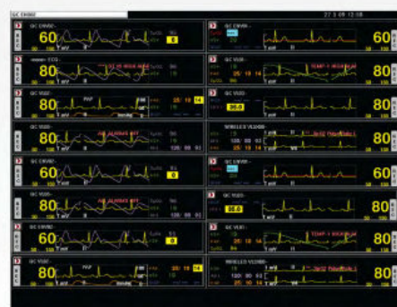
16 monitored beds display showing large HR, vital signs' parameters and two waveforms of each patient bed
