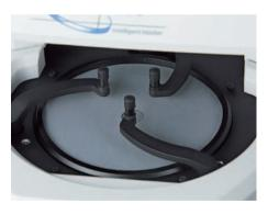
Closed position for lens blocking (multiposition lens stage is motorized)
