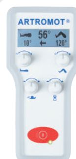
Handheld programming unit ARTROMOT®-K1 classic
