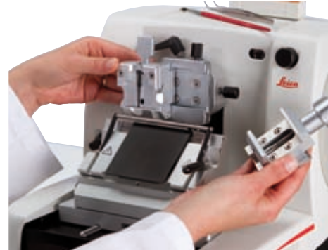
Quick-exchange specimen clamp
