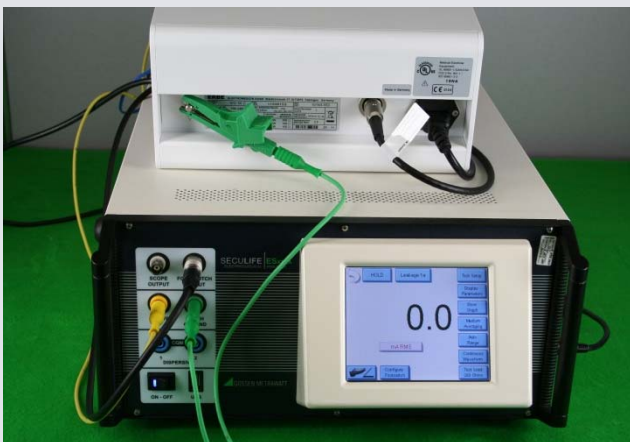
Figure: active output grounded, type CF 1a, e. g. bipolar
