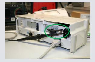
Connection DUT with the SECULIFE ST and connection with the probe
