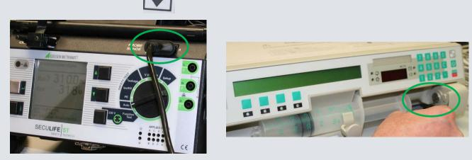
Connection DUT with the SECULIFE ST and connection on the DUT (in this case: infusion pump)
