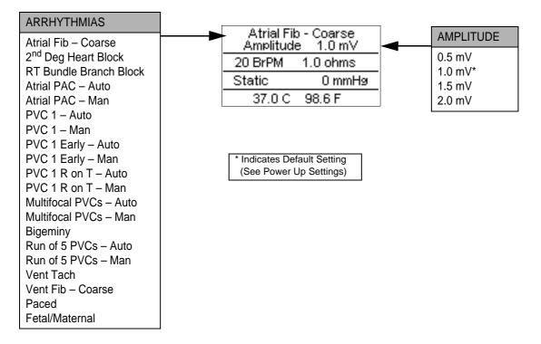
The arrhythmias and amplitude can be selected by using **PREVIOUS NEXT** to highlight the parameter to change and using **UP DOWN** to scroll to the desired value. Then **ENTER** is used to accept the new setting.
