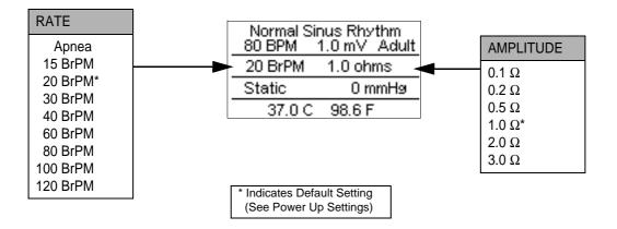
These rates and Impedance Variations can be selected by using **PREVIOUS NEXT** to highlight the parameter to change and using **UP DOWN** to scroll to the desired option. Then **ENTER** is used to accept the new setting.
