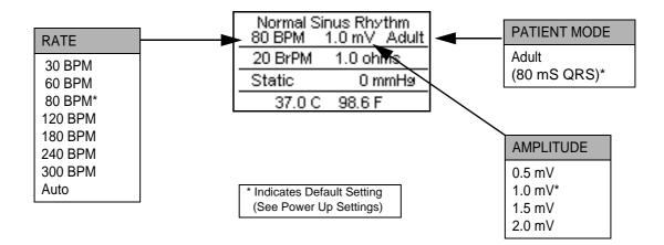
The rates and amplitudes can be selected by using **PREVIOUS NEXT** to highlight the parameter to change and using **UP DOWN** to scroll to the desired value. Then **ENTER** is used to accept the new setting.
