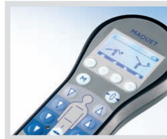
Intuitive operating interface with illuminated keypad area and extensive position memory
