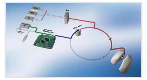
The FLOW-i rebreathing system is optimized with the exclusive VOLUME REFLECTOR which together, with the SERVO-controlled gas modules, enables higher ventilation performance compared with traditional bag-in-bottle and piston-operated systems.
