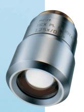
**Leica's special HI PLAN CY 10x/0.25 objectives** feature excellent field flattening and color correction, and offer a long working distance of 12mm. These objectives are also available in an SL (Synchronized Light) version.
