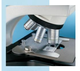
**Quickly change specimens** with Leica's new slide holders, designed so that slides can be changed in a single motion with one hand.
