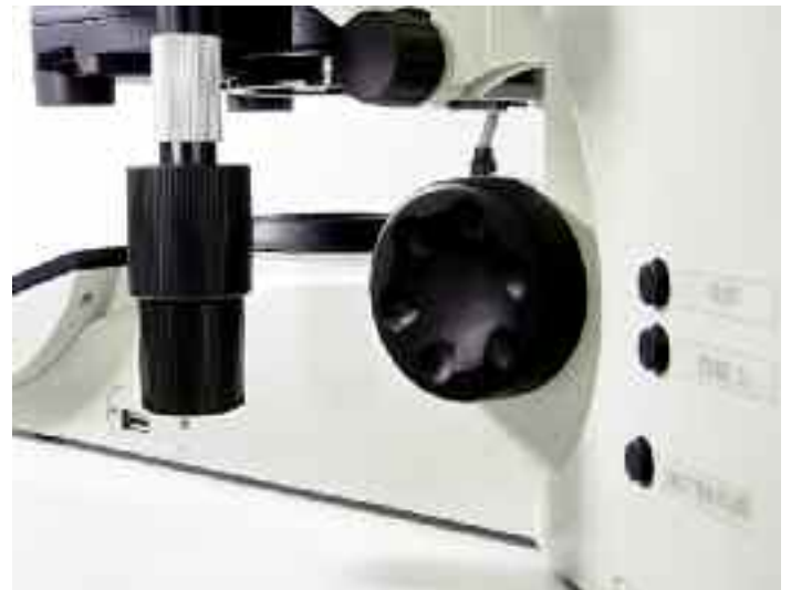
Any desired microscope function can be assigned to the programmable function buttons.
