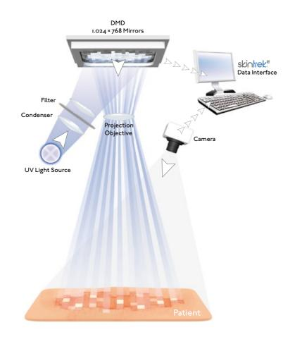
The calculation of the required dose is based on the treatment data of the doctor and the topological information of the skin surface. The topological data is previously calculated in a separate process. This ensures a very precise and accurate dosage of the affected area in comparison with UV-exposure cabins or treatments using UV-lasers. The doctor is able to choose from a multitude of dosage profiles, for example a lower dosage near the edge of a lesion.
