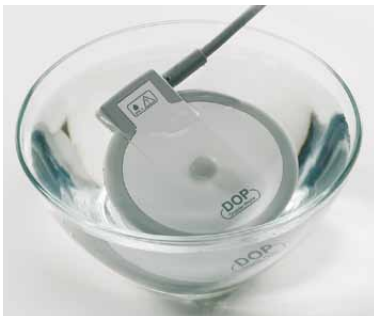
Waterproof transducers with 9 elements
