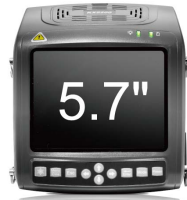
5.7 Inch high resolution colour TFT LCD monitor forming a clear image under the sunshine for special treatment.
